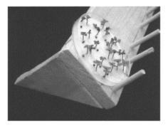
**FIGURE 12.1** Wooden apparatus for holding petri plates at a 45° angle. (Courtesy of B.R.Cody North Carolina State University.)
